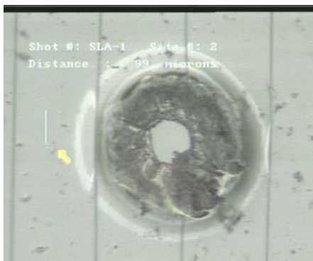
Figure 11. Sample after Hypervelocity shot
