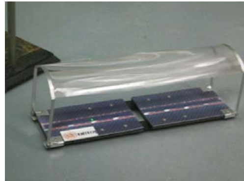
Figure 13. Picture of wind distortion to lens with light remaining focused on cells
