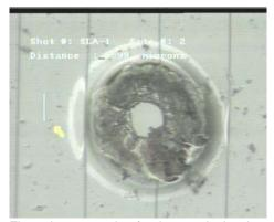
Fig. 6. Lens sample after hypervelocity shot
