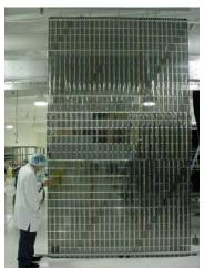
Fig. 3. A 3.75 kW Stretched lens array on a SquareRigger platform
