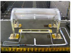
Fig. 7. SLATE-T4 Parquet-Coated Lens and Three-Cell Photovoltaic Receiver Mounted on TacSat IV Solar Array Panel
