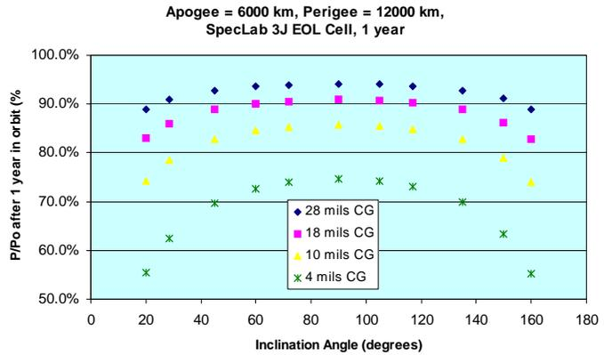
**Figure 3.** Power degradation of solar cell as a function of inclination angle and cover glass thickness
