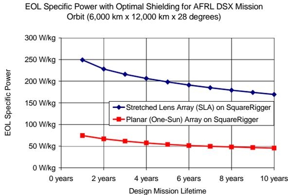
**Figure 4.** EOL Specific Power Comparison
