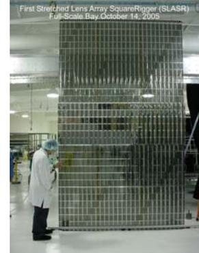
**Figure 1.** Full scale SLASR module
