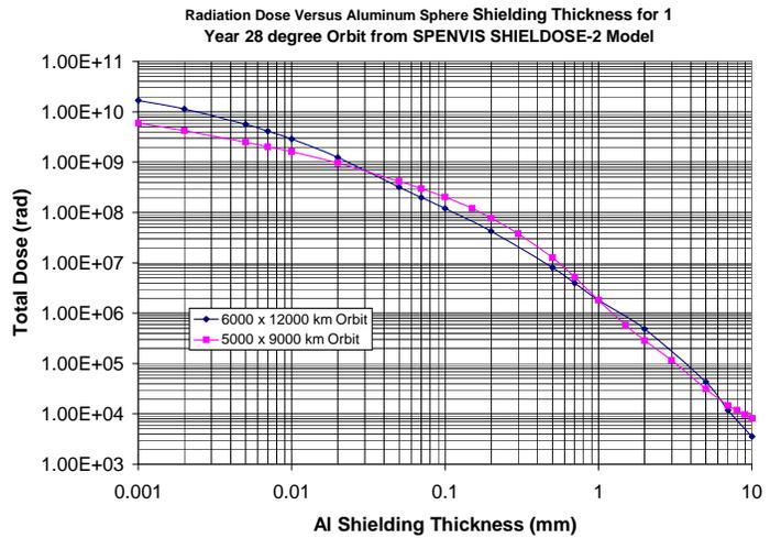
**Figure 6:** Total Dose versus shielding thickness
