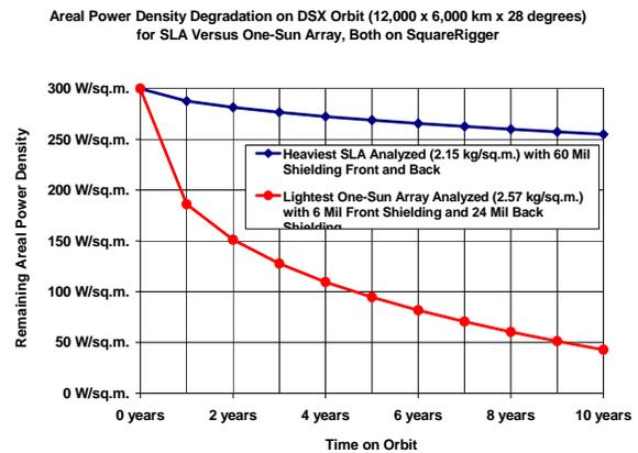
**Figure 5.** EOL Areal Power Density Comparison
