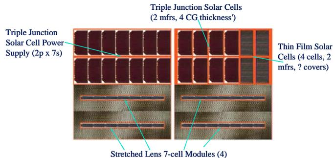
**Figure 2.** Preliminary Design of SLATE
