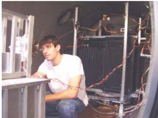
Fig. 15: Auburn student inspects Russian T-100 thruster
