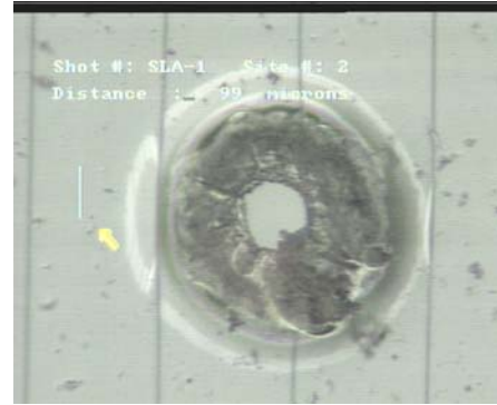
Figure 10 - Sample after Hypervelocity shot
