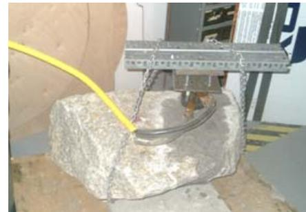
**Figure 11. Granite rock, approx  $0.085 \text{ m}^3$  ( $3 \text{ ft}^3$ ) ready to be blasted.**
