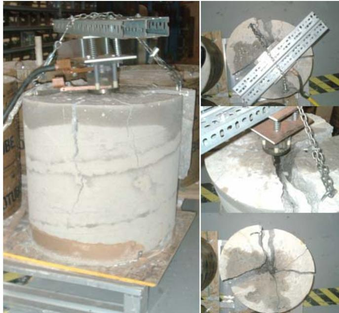
**Figure 10. Concrete Sample,  $0.075 \text{ m}^3$  ( $2.65 \text{ ft}^3$ ), after blast with a charging voltage of 11 kV.**
