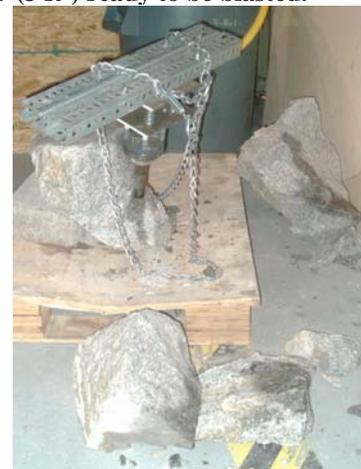
**Figure 12. Granite rock after plasma blasting.**
