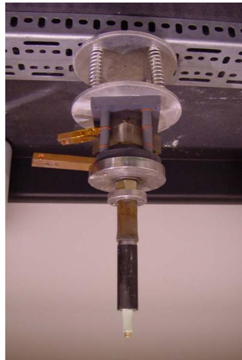
**Figure 3. Plasma Blasting Probe**
