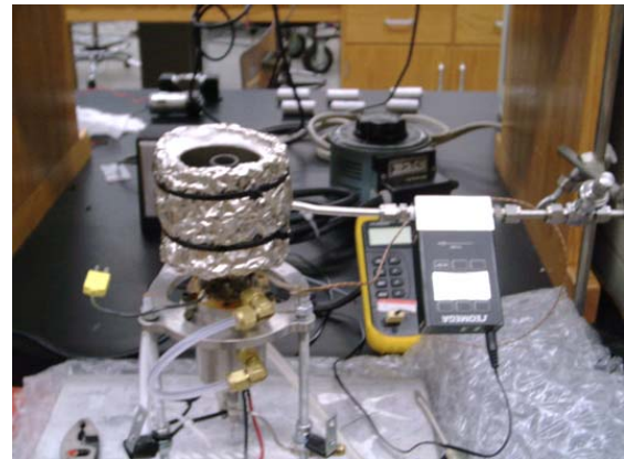
Figure 9. H 2 Burner coupled to a 35We FPSE
