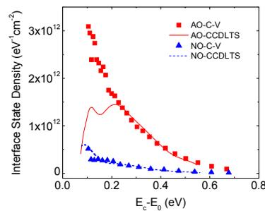
Fig. 4.  $D_{it}$  determined from Hi-Lo C-V and CCDLTS measurements.
