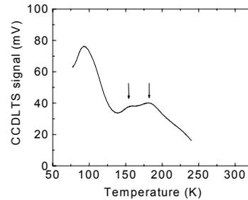
Fig. 2. Saturated CCDLTS spectrum for an NO sample. The rate window is 8.6ms.
