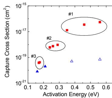
Fig. 3. Capture cross section vs. emission activation energy for AO and NO samples.
