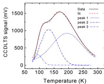
Fig. 1 Saturated CCDLTS spectrum for an AO sample. The rate window is 8.6ms. Data are fit as the sum of three trap distributions.
