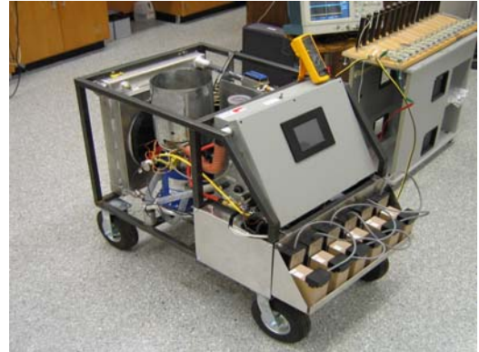
FIGURE 5. Stand-Alone, 1.2 kW Stirling Convertor Battery-Charging Power System.
