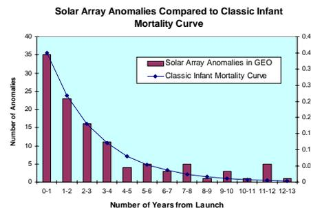
Fig. 2 Solar array failure trend showing a classic infant mortality profile
