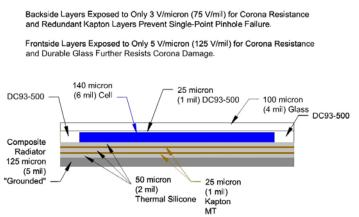
Figure 6 - Test sample configuration
