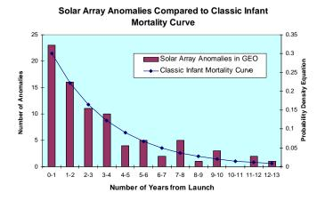
Figure 4 - Years b/w launch and solar array anomaly in GEO
