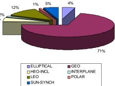
Figure 2 - Solar Array Anomalies by Orbit 1996-2006
