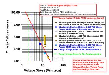
Figure 7 – Results of underwater hi-pot testing
