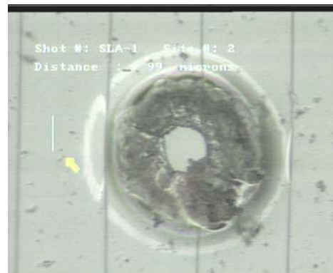
Figure 4: Lens sample after hypervelocity shot
