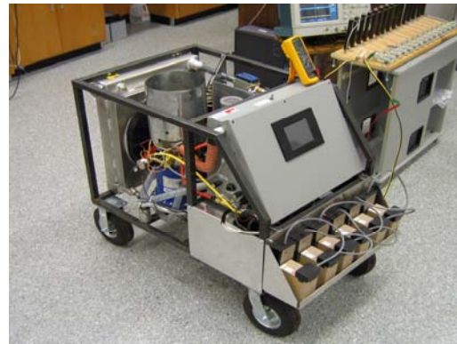
Figure 5. Stand-Alone, 1.2 kW Stirling Convertor Battery Charging Power System.
