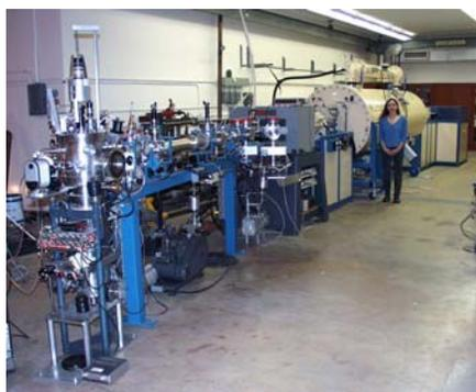
Figure 2: NEC Pellatron 2 MV Dual Source Tandem Accelerator
