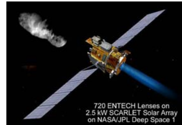
Figure 2: SCARLET array on NASA/JPL Deep Space 1 probe (1998-2001).
