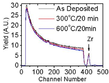
FIG. 3. (Color online) Rutherford backscattering spectroscopy of the  $\text{ZrB}_2/\text{GaN}$  contact.
